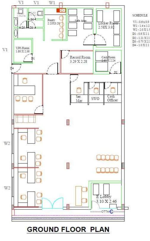
V1-0.6x0.9 W1 - 1.4 x 1.2 W2 - 2.0 X 1.5 D1-09X21 D2 - 1.21 X 2.1 D3 - 0.75 X 2.1
