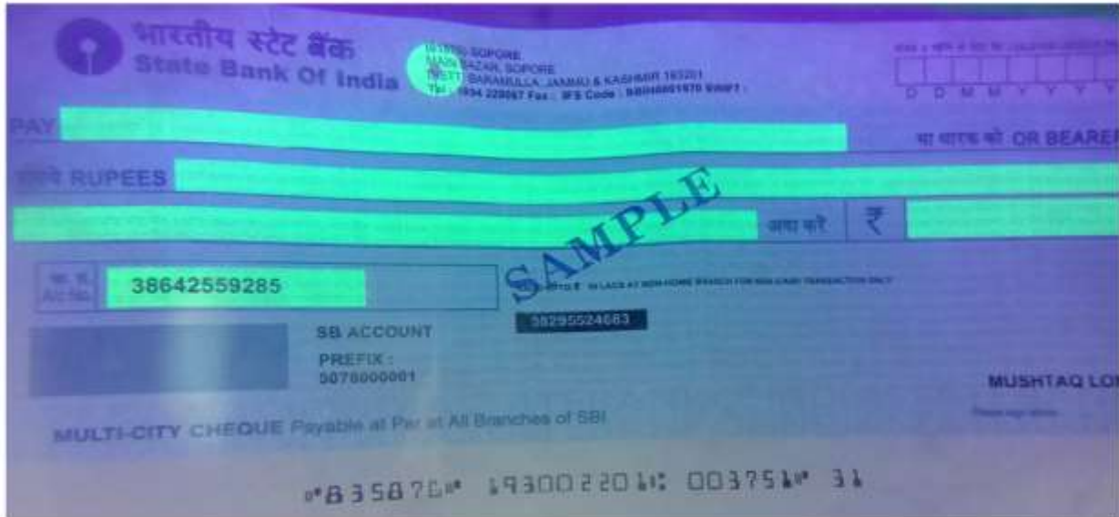
Area highlighted are covered under UV ink and can be seen under UV lamp.
