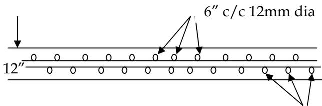
Where it is not feasible to provide R.C.C. slab 6" c/c 12mm dia reinforcement should be fortified with M.S. grills consisting of 20 mm rods spaced 75 mm centre to centre in angle iron frame work.
